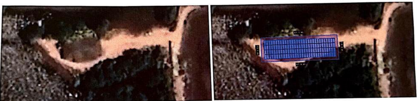
Preliminary design of solar panel layout (New structure with 3m height)
